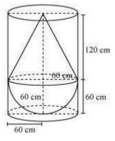
Radius (r) of hemispherical part = Radius (r) of conical part = 60 cm
