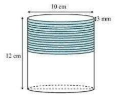
It can be observed that 1 round of wire will cover 3 mm height of cylinder.
